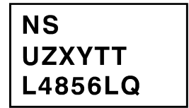
Top View NS - Std NS Logo U - Wafer Fab Code Z - Assembly Plant Code XY - 2 Digit Date Code TT - Die Run Traceability L4856LQ - LM4856LQ
